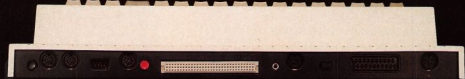
Break Button MIDI in Mouse Expansion Connector Light Pen/Gun SCART socket MIDI Out Joystick Reset Button Cassette On/Off Switch Power/TV
