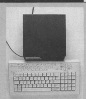
Opus Discovery — probably the most popular Spectrum disk drive. And rightly so. The unit contains a 256K 3.5-inch disk drive, parallel printer port, joystick port, video socket and a power supply for both itself and the Spectrum. An on/off switch is a useful bonus too.
