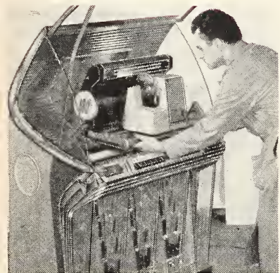
Entire mechanism slides out from front and rests on selector castings for easy cleaning and servicing.
