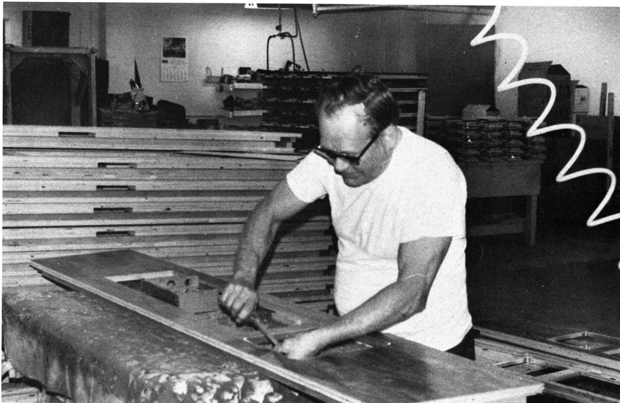
In another step in the final assembly area, a worker affixes the metal trim to the interior moldings.
