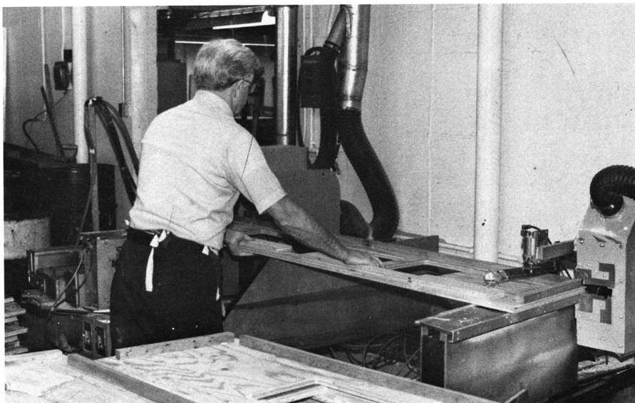
A worker handles the cutting and assembly of one of the table's side panels.
