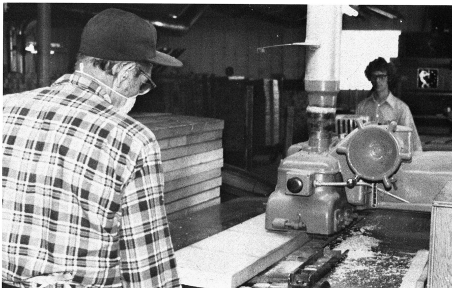
Two Valley workers slide boards through the width cutter to one another in the process of modifying raw materials to Valley's table specifications.
