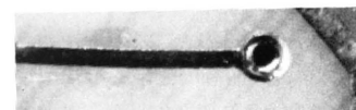
AFTER REPAIR with SRS-050 Kit, the Pad and Eyelet have been neatly replaced.
