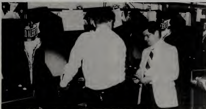
RIGID TESTING — GDI quality control inspectors are shown testing "Red Alert," the firm's first entry in the video game market, after a 24-hour burn-in period.
