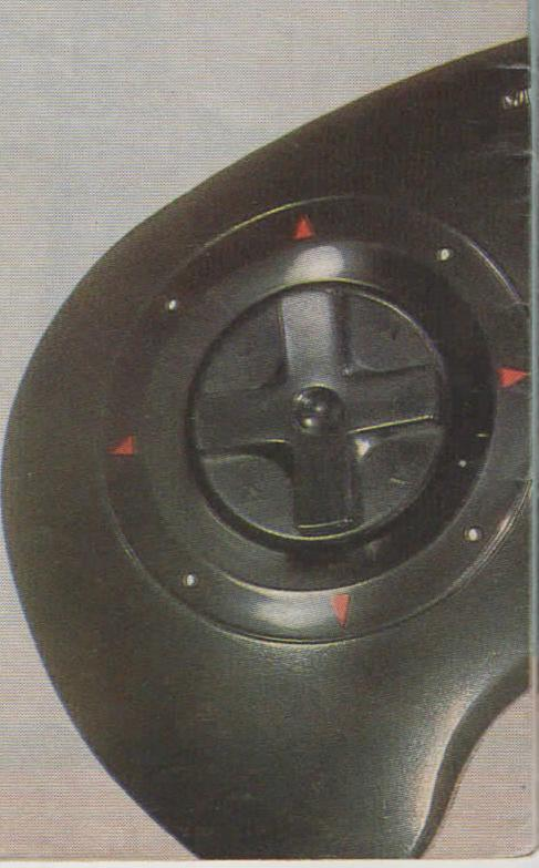
The MEGA DRIVE system comes with a flat crescent shaped joypad in which is housed a Start button, three Fire buttons and a Directional (control) pad. Reacting well to vigorous playing the Directional pad does not have the stiffness usually associated with this type of controller which makes diagonals easier and faster to reach. The joypad is plugged in via a D-type connector which makes using Turbo Control pads or Joysticks possible.
