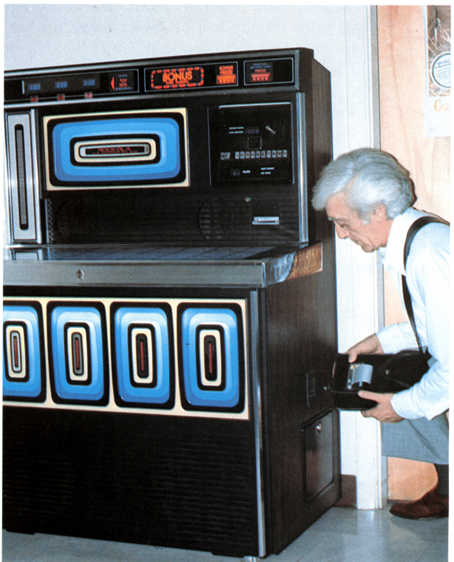
The interrogating printer reads the LED display on each machine to give an accurate report on how many times the coin switch was tripped.
