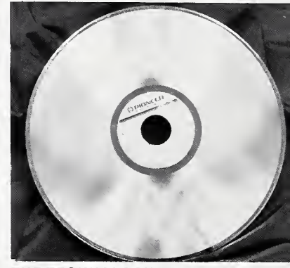
THE TECHNOLOGY — Resting above is a sample laser disc containing all of the software animation to "Space Ace." It is the random access capabilities of this unique storage device that allow the player to interact with different scenes from the game.
