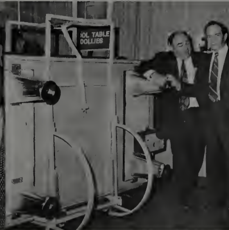
The now-legendary Langhausen pool table dolly, showing its roll-bars (which reportedly enables a single serviceman to install or move a table) got a good looksee by Johnny Bilotta.
