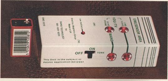
The Electro Magnetic Gauge (above) is new gadget aimed at discovering how much low frequency electro magnetic radiation your computer throws out.
