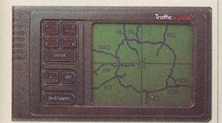
The screen maps out where traffic problems are and alternative routes to take. which delays on motorways and arterial roads begin to happen. The speed shown on the in-car display is an average taken over the three previous minutes and the manufacturer claims it is an average speed that one can expect to get through the delay rather than at a constant speed.
