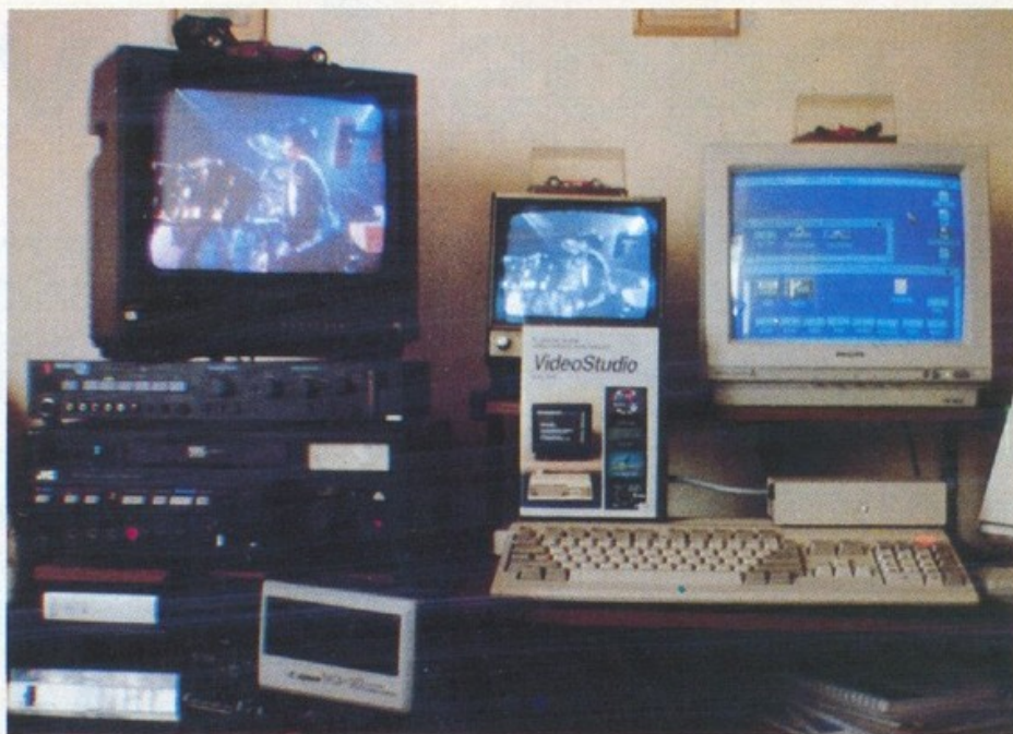
Our reviewer's complete titling set-up with two video recorders and TV/monitors, video camera, Genlock and Amiga with monitor.
