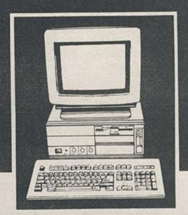
This is an American system switchable between 8-16Mhz. Comes fully configured and desk ready. Fully documented, 2 years all parts and labour warranty. The mother board will take up to 4 Meg of RAM on board with the capacity to take 16Meg on a daughter board. The system is 0 wait state and has 8 slots, 6 being free for expansion. The hard drive is a Western Digital 40 Meg sub 25ms IDE device. The video card is a 16 Bit paradise card 256K populated.
