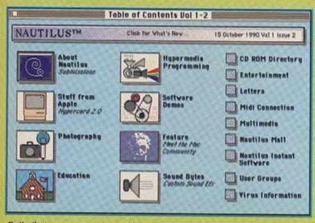
The Nautilus 'contents page' - a Supercard front-end with clickable buttons which launch sub-applications.
