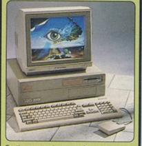
For the more serious or professional applicaror the more serious or professional applica-tions user, Commodore have a selection of systems based around the expandable Amiga 2000, at prices from £1295+VAT. The A2000 features a full 1Mb RAM (expandable to 9Mb), 9 system expansion slots, plus IBM com-patibility with the use of PC-XT or PC-AT bridgeboards. Complete and return the coupon, putting a tick in the A2000 box, for details of A2000 computer systems.
