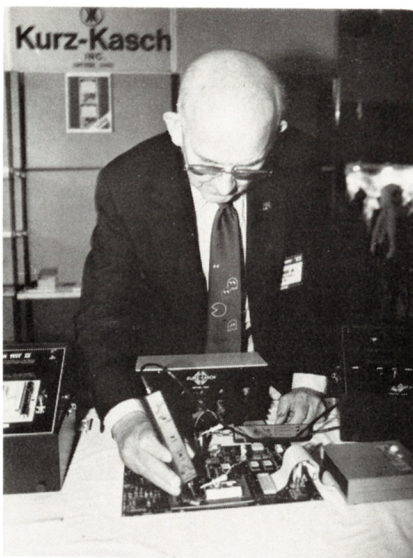
Jim Sneed of Kurz-Kasch demonstrates the use of signature analysis for troubleshooting logic boards.
