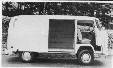
VW VAN: The 1971 Volkswagen delivery van, shown here, features a 60 - horsepower engine, power - assisted braking, and large sliding door on the right side. Options include doors on both sides, or on the left side.
