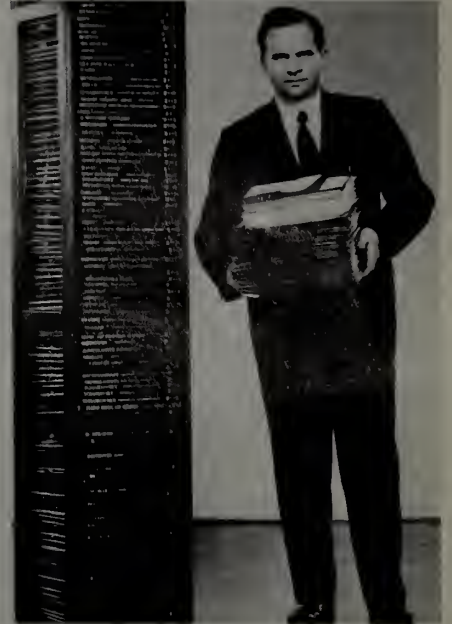
A REVOLUTIONARY FEAT — In this 1948 photograph, the late Dr. Peter Goldmark, who developed the original LP technology, dramatically demonstrated the compactness of 33 1/3 rpm records by standing next to column of 78s, while holding an equal duration of music in his arms on long playing discs.
