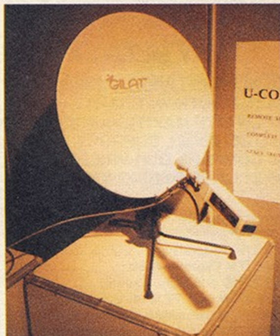
• Gilat's U-Cord system - a receive-only terminal for data communications able to incorporate different satellites and antenna diameters and capable of handling up to 112Kb per second of data. Prices for this remote terminal start at £800.
