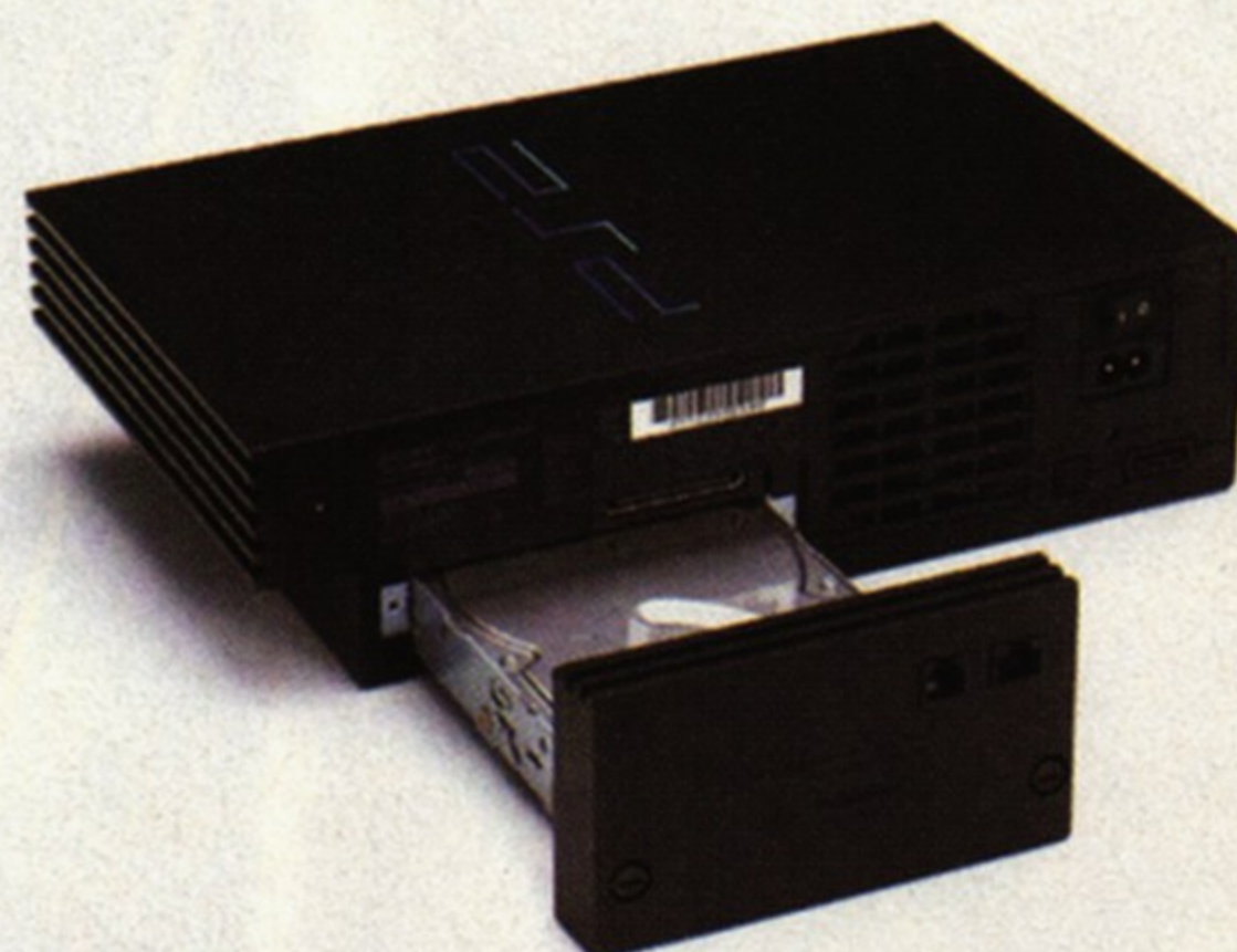
The hard drive, which will be released in November, slides into the expansion bay of the PlayStation 2.
