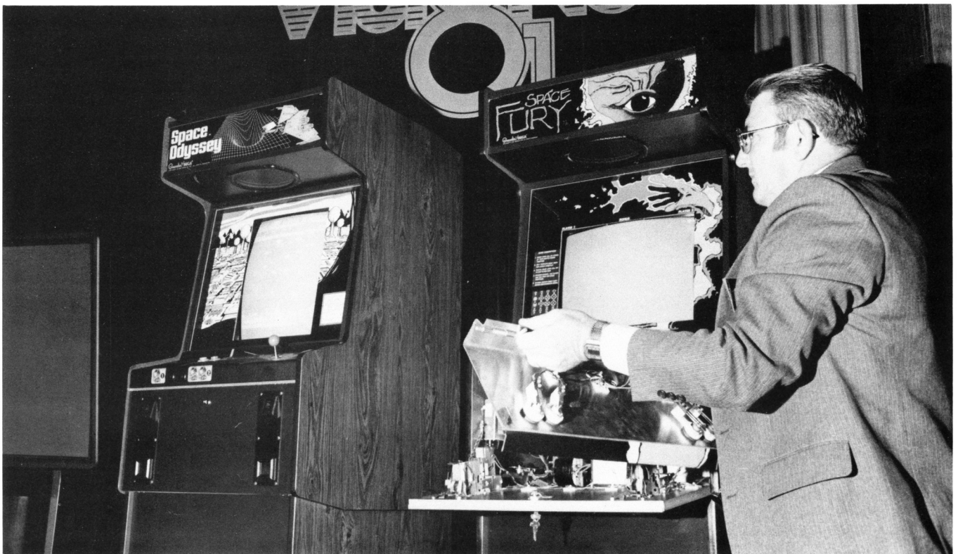
Changing of PC boards within 15 minutes with the Convert-A-Game system is demonstrated by a Sega engineer at a recent showing for handlers.
