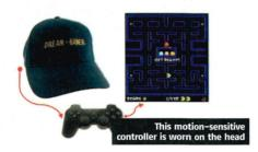
controller to make it possible to use. The Dream-Gamer is one such device. It's a cap fitted with motion sensors that detect the movements of the wearer's head.
