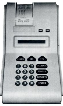
Surprise! The clerk validation terminal (CVT) is not a mysterious "black box." It's actually a white box with blue and orange buttons, a display screen, and a microprocessor inside. It can validate tickets plus print out other important data.
