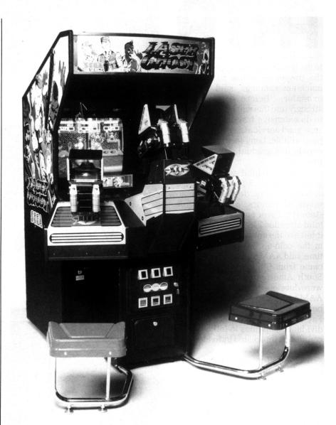
technology that we've used before and found highly reliable." The three guns are also anchored firmly in place; there's no chain or cable to twist or break. As Tom Petit put it: "They're not going anywhere!"
