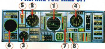
1) ARTIFICIAL HORIZON: One of the most important instruments. Its function is to indicate the roll and pitch of the aircraft, relative to the horizon.
