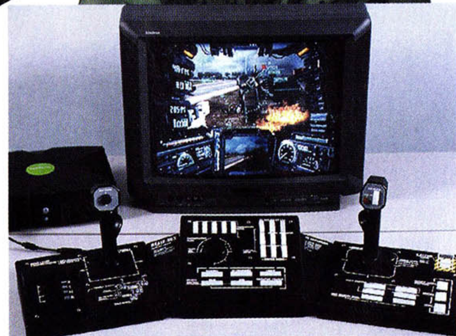
The Steel Battalion controller (which comes packaged with the game) features 40 buttons, flashing lights, two joysticks, a tuning dial, and three foot pedals
