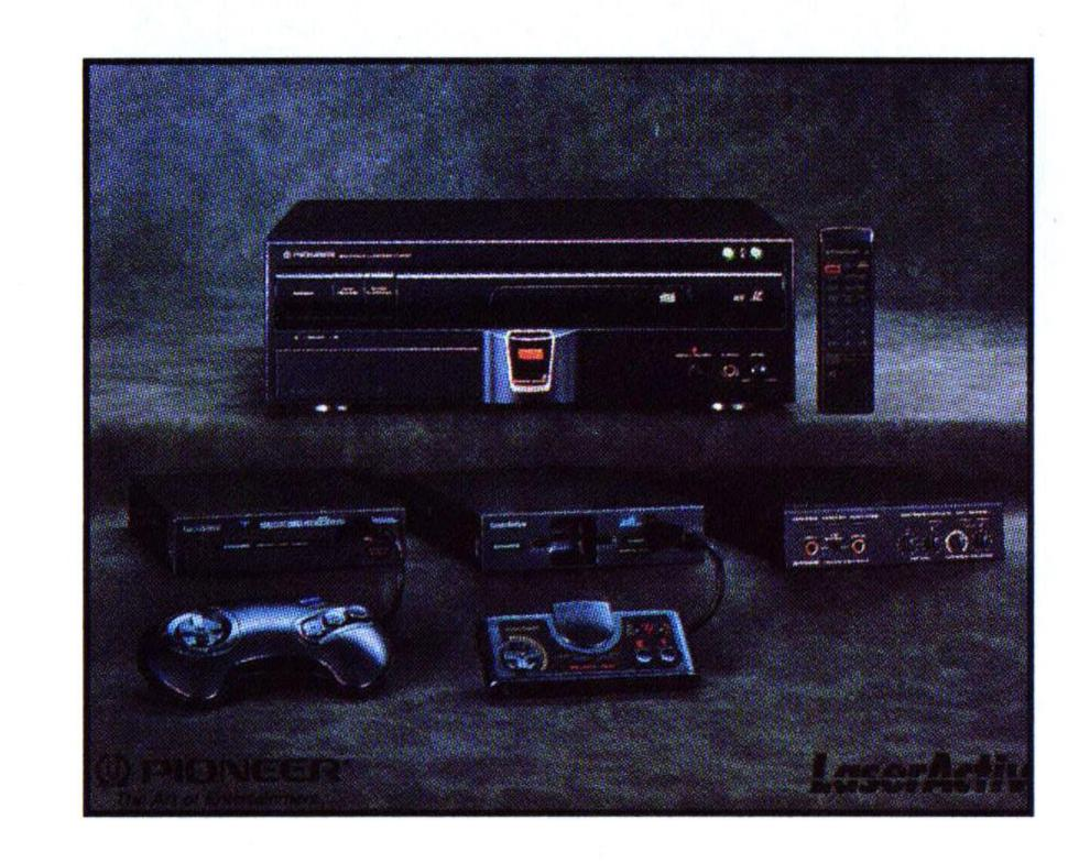
create optional control packs for the *LaserActive*. The Mega-LD<sup>TM</sup> plays 8-and 12-inch *LaserActive* Mega-LD discs, Sega CDs, Sega Genesis ROM cartridges and standard CD-Gs. The LD-ROM<sup>2</sup>TM, developed in cooperation with NEC, plays 8- and 12-inch *LaserActive* LD-ROM<sup>2</sup> discs, TurboGrafx CDs and ROM cards, and standard CD-Gs. A third *LaserKaraoke*<sup>TM</sup> pack is compatible with *LaserKaraoke* discs and standard CDs.
