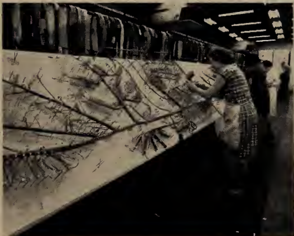
Miles and miles of intricate electrical wiring are secured and coordinated by the ladies on the lines. They are part of the 700 Williams employees working in the factory.
