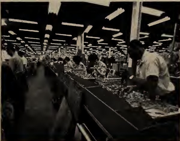
Checks and counterchecks on coin chutes and moving parts are made by these workers. Each worker gives each part close inspection to assure that the finished games are trouble-free when shipped and on location.
