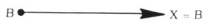
Fig. 4-18. The simplification of the circuit in fig. 4-17. Notice that all gates were redundant and the entire circuit was replaced with a conductor.
