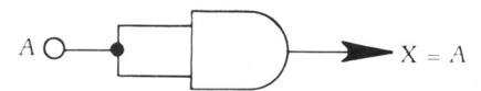
Fig. 4-9. Both inputs of an AND gate connected together. This circuit demonstrates the Boolean expression A \times A = A .
