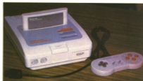
Notice that the Super Nintendo controller has four fire buttons rather than the usual two.
