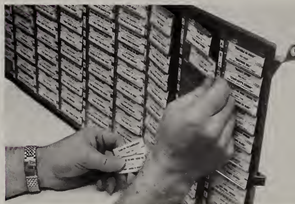
Patented "flip-out" plastic racks allow simple, one-hand title panel service . . . entire panel swings free for easy service.
