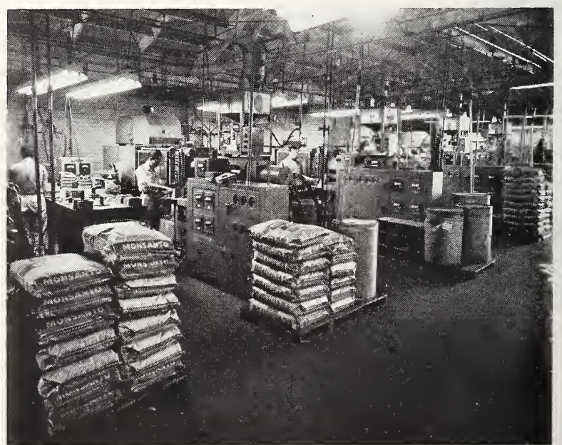
4. Automatic injection molding factory where phonograph records and toys are manufactured.
