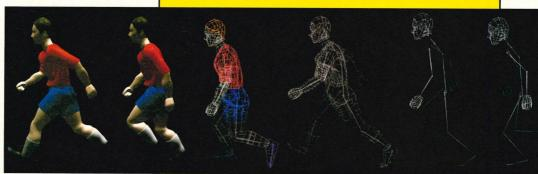
These show how the sprites in FIFA were put together. They begin as simple line drawings, and the polygons are gradually built on.
