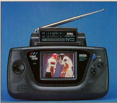
Expected to retail for about $149.95, the Game Gear has a screen resolution of 160 x 146 pixels and can display 32 colors at a time out of a palette of 4,096.
