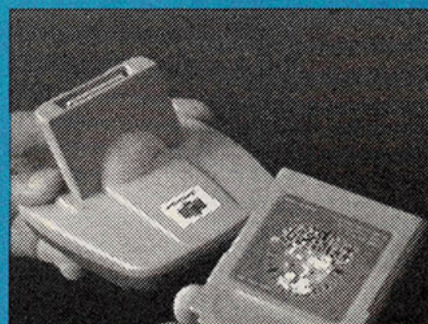
8-bit and 64-bit Pocket Monster games can coexist with the help of this special Game Boy adapter for the Nintendo 64 controller.
