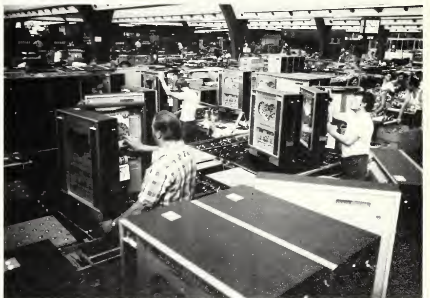
PRODUCTION LINE — A portion of one of the numerous assembly lines in the Lowen factory complex. Considerable space at the facilities is allotted to imported products from the U.S. and other countries throughout the world. In this photo, workers are assembling the firm's popular Rotamint amusement machine.
