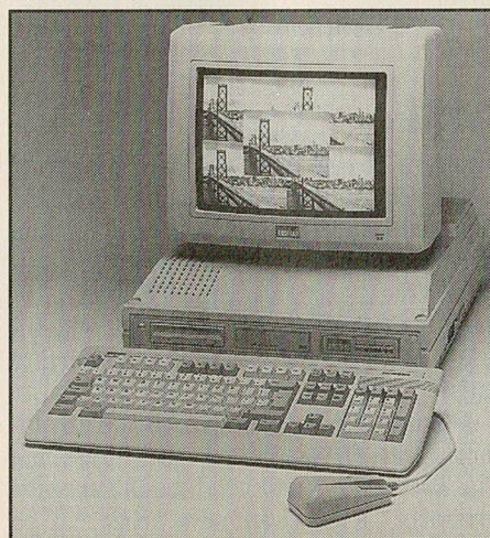
Amstrad PC 2386: features 20 MHz Intel 80386 MPU and 65 Mb hard disc.
