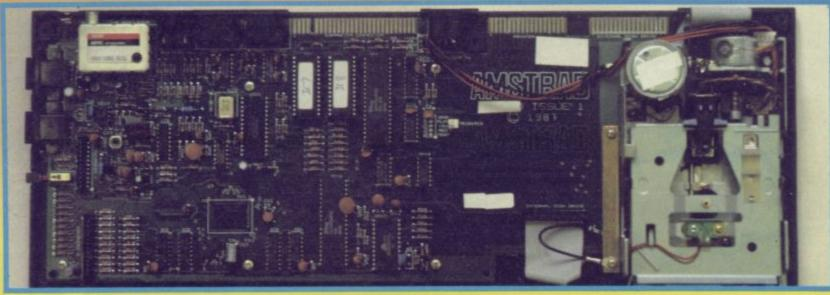
horror – the Plus 3 isn't Interface 1 and Microdrive compatible. You can plug in Interface 1, but it won't work. The reason lies buried deep in the Plus 3 hardware, so it's not going to be possible to produce a software fix.
