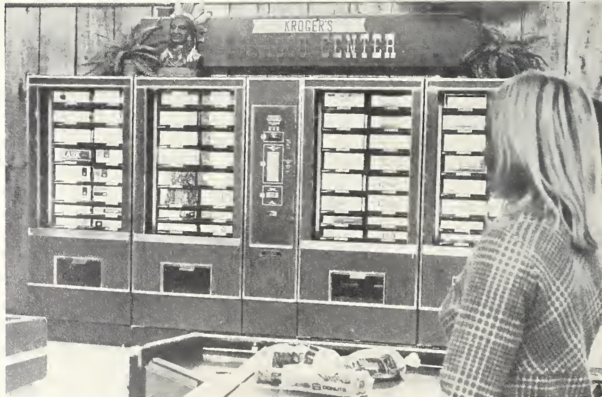
National's Golden Showcase, shown above in four dispensing module bank, operates on a card-validation system.
