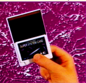
The PC Engine Super System Card needs a special adapter to work with the Turbo-CD.
