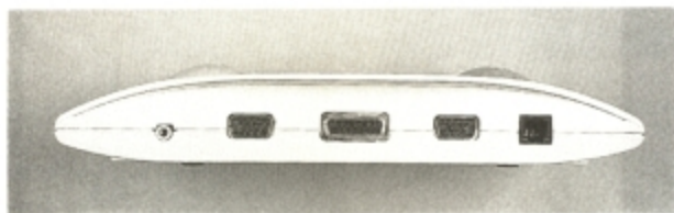
From left to right: stereo phono socket, player 1 joypad/joystick connector, analogue joystick port (accepts two sticks with suitable adaptor), player 2 joypad/joystick connector, auxiliary port for light gun.
