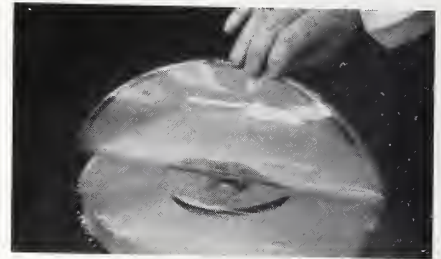
Technician removes a videodisk replica from replicating machine.
