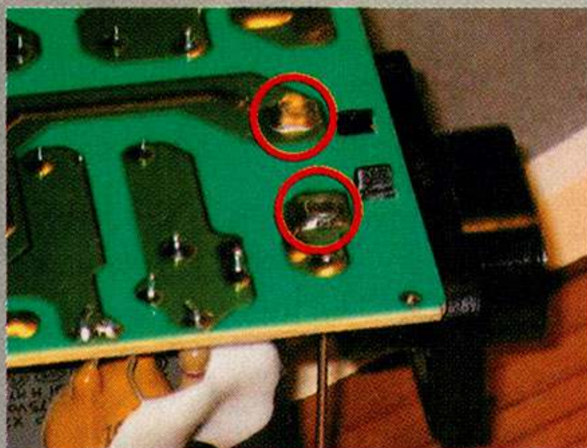
With only two soldering joints, the connector for the Foxlink PSU can easily become loose, putting it at risk of burnout or electrical sparks.
