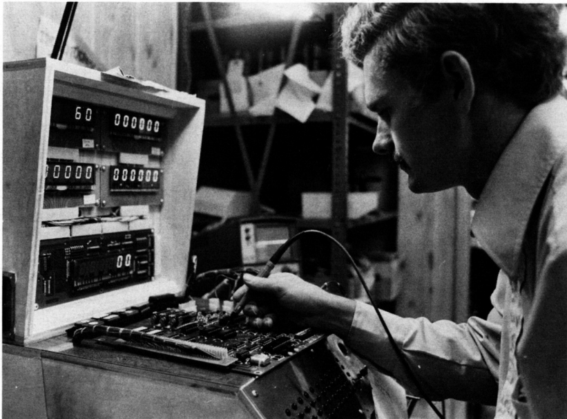
The all-important digital scoring displays—where all eyes focus as bonus points ring up—are tested for accuracy by a Williams Electronics, Inc. technician at the firm's Chicago factory, one facet of Williams' efforts to ensure quality production.
