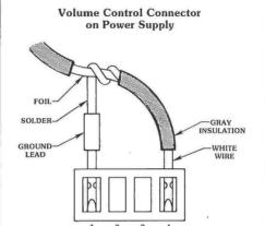
Be careful not to strip away the foil underneath. Make a small jumper
