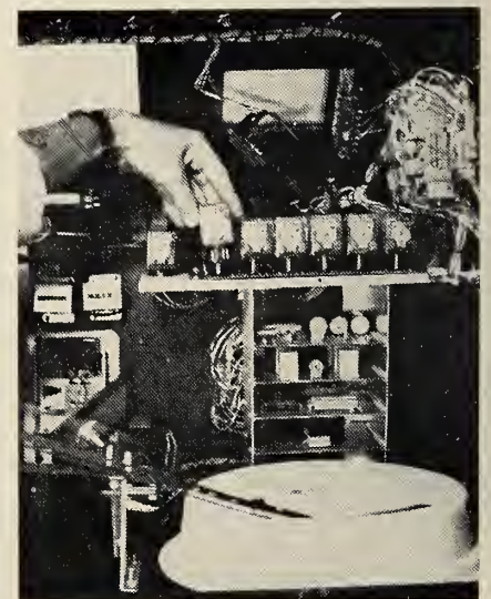
Here the hand is holding one of 13 plug-in relays. The white space above the hand is the screen where the questions are projected from a film strip being fed thru the larger circular disc at the bottom of the photo.
