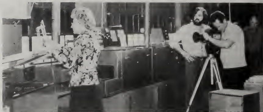
INSIDE LOOK — The Rock-Ola phonograph manufacturing plant was featured recently on the NBC-TV program "Bubble Gum Digest." In the above photo, the television cameras zoom in on an employee who stands before a vat of molten solder through which printed circuit boards float. Chemically treated areas on the bottom of the boards accept the solder and complete the circuits.
