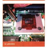
the point of contact. If not, clean off any existing thermal compound and add a small amount of fresh material.
