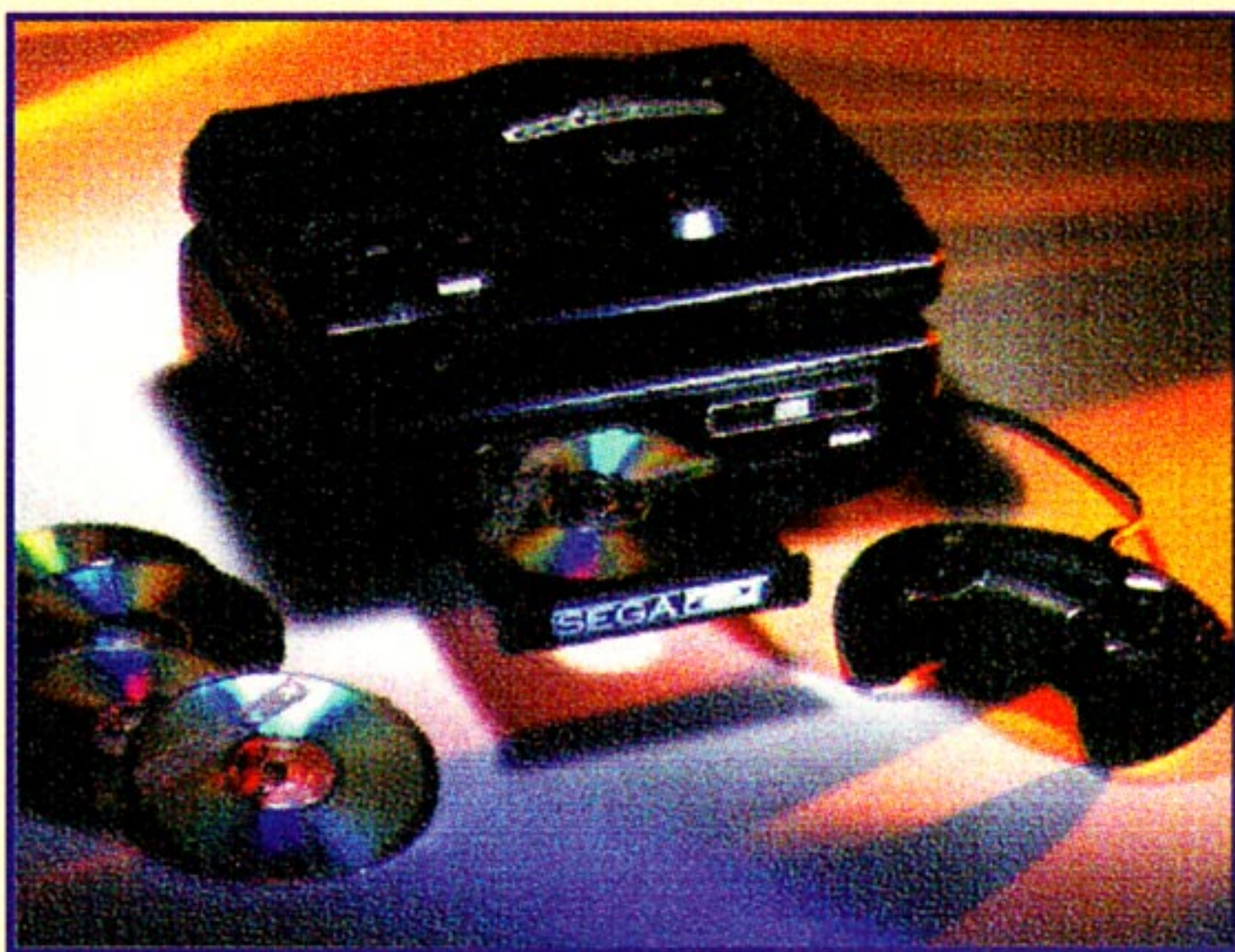
The Sega CD allows the use of Genesis carts as well as multimedia CD titles.
