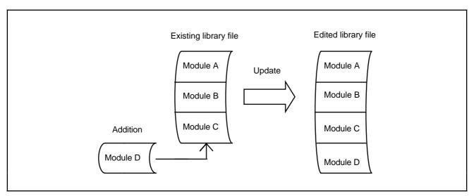
Figure 2-2. Adding a Module
