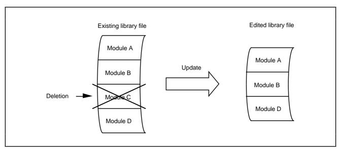
Figure 2-3. Deleting a Module
