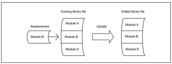
Figure 2-4. Replacing a Module
