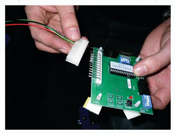
4. Connect the 10 way edge connector to the Excel credit board as shown in the picture.
