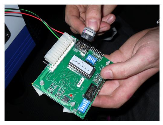
5. Connect the 10 way coin loom into the excel credit board. N.B. It must be connected to CN5 input
