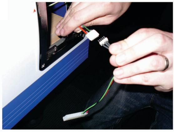
3. Connect the 10 way edge connector of loom supplied, to the loom from the original coin mechanism. Note that the colours should match pin to pin.
