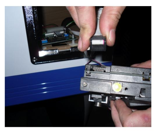
6. Connect the other end of the 10 way coin loom to the SR3 coin mechanism
