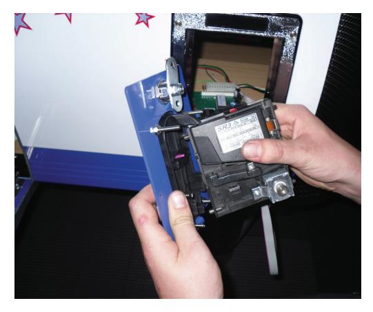
7. Clip the SR3 coin mechanism into the faceplate.
