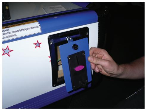
Open door and disconnect coin loom and remove original mech (2 screws) and face plate.
