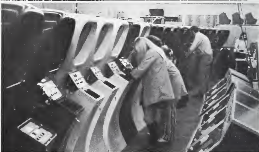
Computer Space machines on the Nutting Associates assembly line are getting the final tests.
